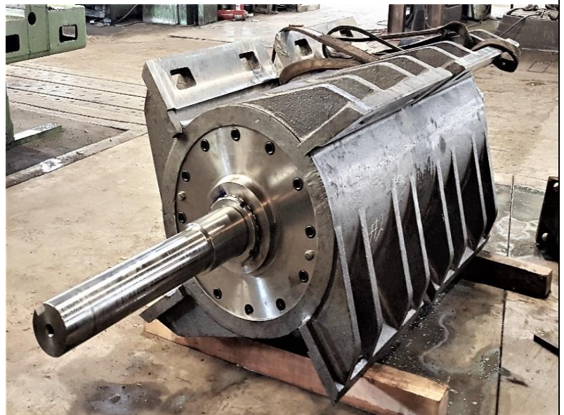
Reverse-Engineered Rock Crusher with Shaft
